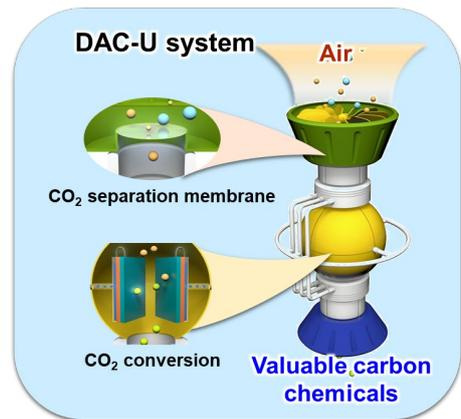
The Direct Air Capture and Utilization System (DAC-U®) has a separation membrane acts like an air filter to capture and condense CO<sub>2</sub> from the atmosphere and convert the CO<sub>2</sub> into other useful substances.
